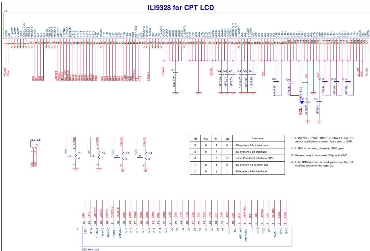
1. If VSYNC, HSYNC, DOTCLK, ENABLE and SDO are not used, please connect these pins to GND.
