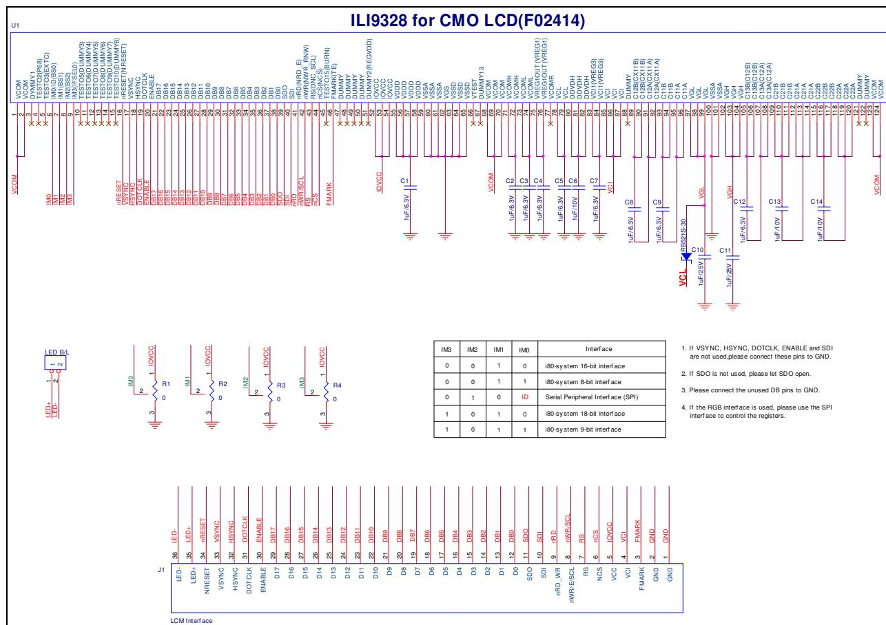
1. If VSYNC, HSYNC, DOTCLK, ENABLE and SDI are not used, please connect these pins to GND.
